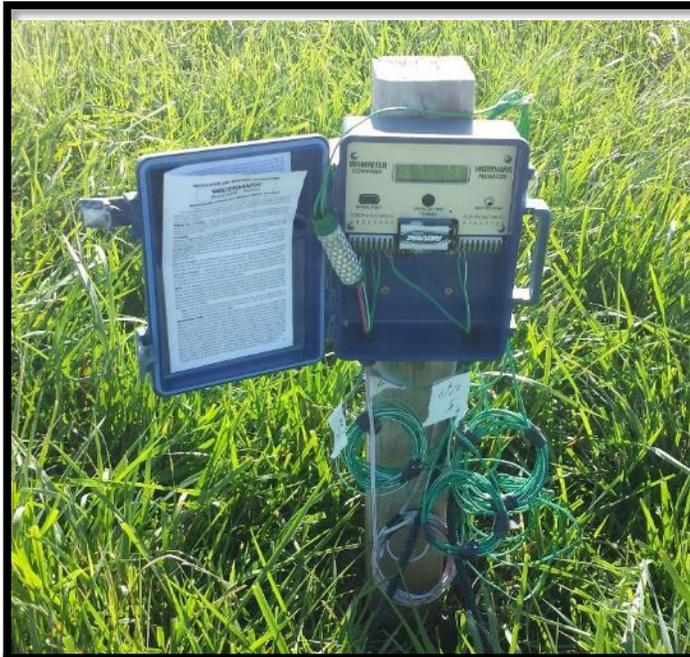
**Figure 2.** Automated Soil Moisture Recording Device for Watermark™ Sensors.
