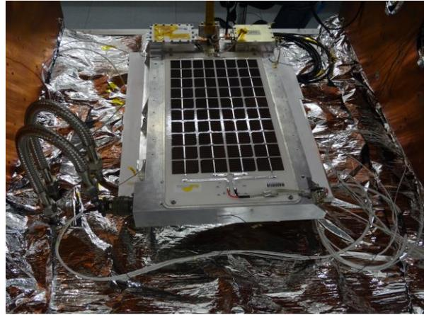
**Figure 2: 4M in thermal vacuum chamber for thermal vacuum test and activation sequence test**
