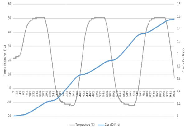
**Figure 3: Temperature log of thermal vacuum test and corresponding clock drift**
