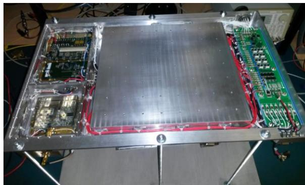
**Figure 1: 4M spacecraft upside down with open bottom**
