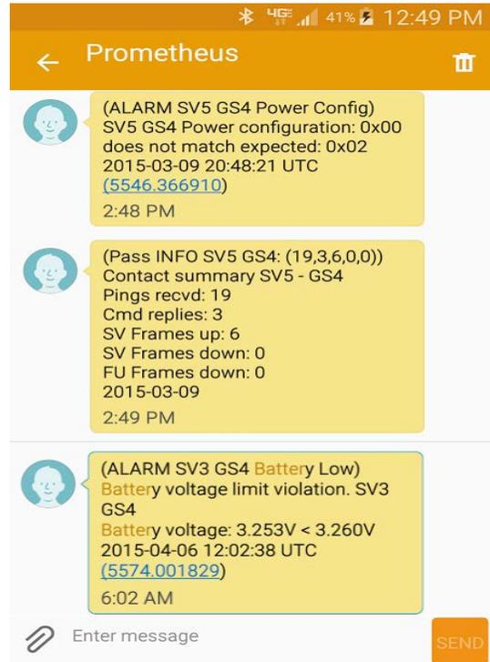
**Figure 8: Text Messages Showing Alarm and Status sent from Prometheus Ground Station**
