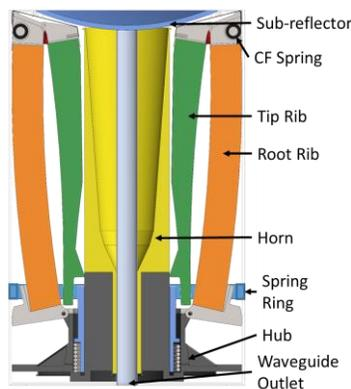
Figure 3: Key KaPDA Components
