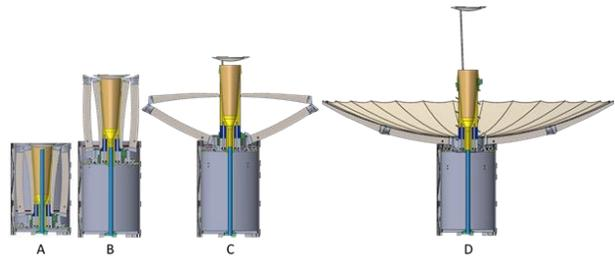
Figure 4: KaPDA Deployment Sequence
