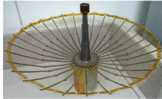
**Figure 1: Aeneas Spacecraft was the first high gain CubeSat antenna to fly**
