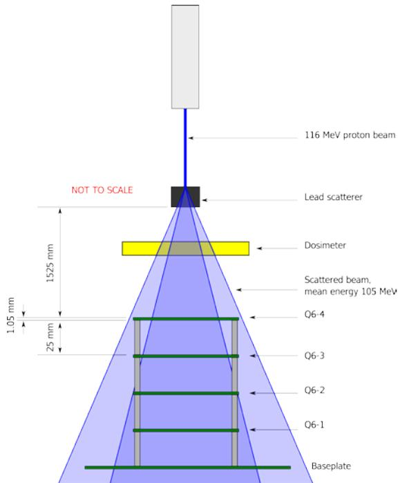
**Figure 2: Radiation Exposure Configuration**
