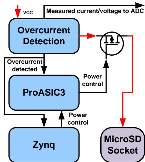
Figure 4 Q7 MicroSD Over-Current Protection
