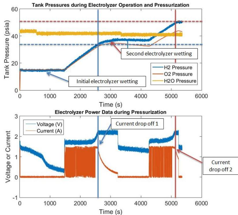
Figure 3. Electrolyzer Performance with Additional Wetting
