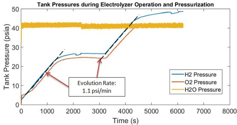
**Figure 4. Electrolyzer Gas Generation Rates**
