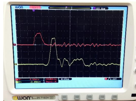
Figure 7: Low Side Driver Test Output
