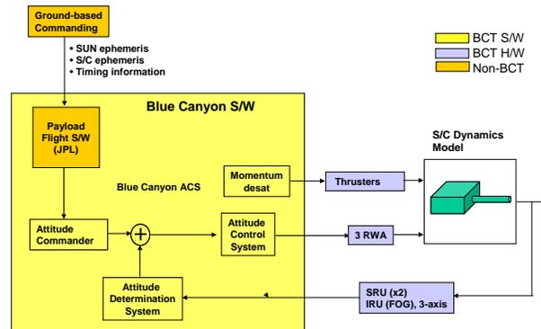
**Figure 9. Block diagram of the MiniCOR ACS system.**
