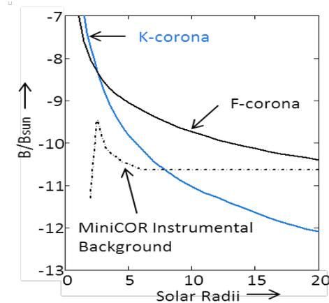
**Figure 6: The brightness profiles, in units of mean solar brightness, of the unvignetted K-corona, F-corona, and the MiniCOR maximum expected instrumental background over the 2.5 $R_s$  to 20 $R_s$  field of view are shown. The stray light will be below the modeled background.**
