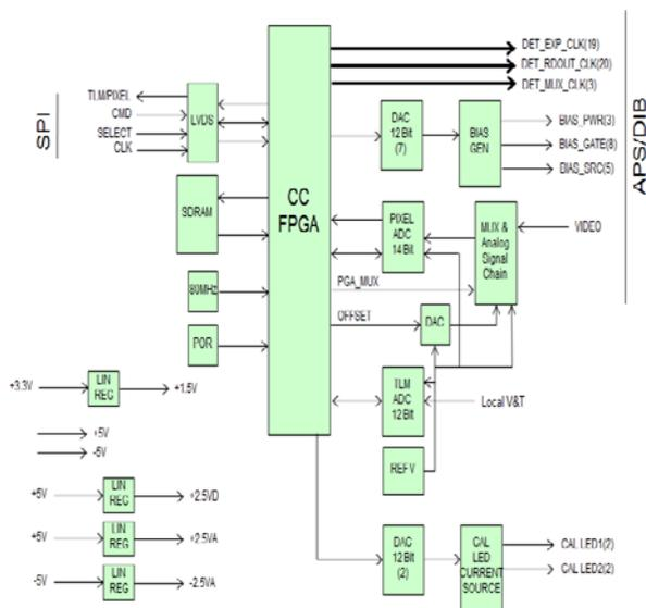
**Figure 8. Block diagram of the MiniCOR camera electronics. The functionality of this card is very similar to the WISPR camera electronics presently under development at NRL.**
