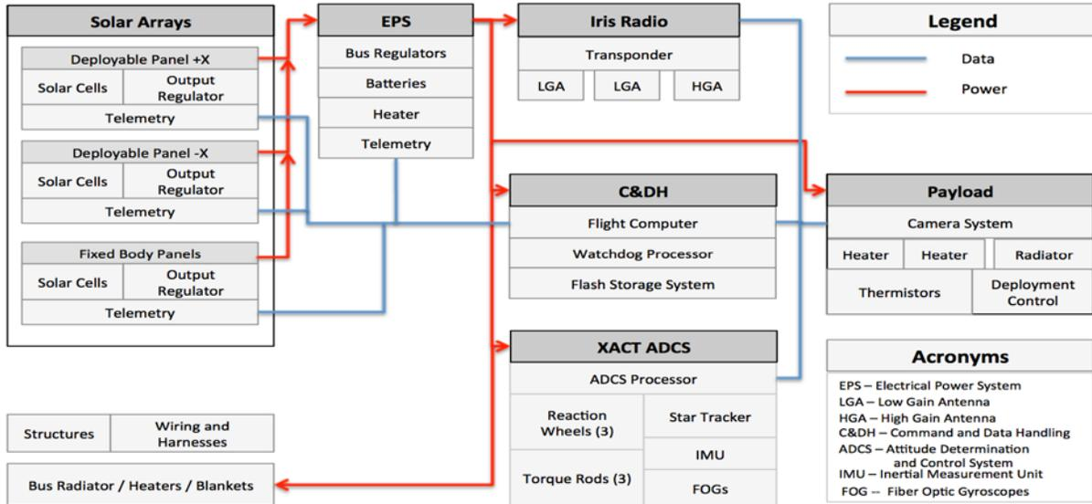
Figure 3. MiniCOR block diagram
