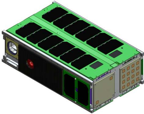
**Figure 10: HGA patch antenna array and LG “receive” and transmit antennae at the rear of the spacecraft.**
