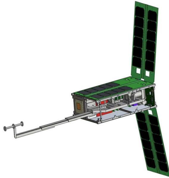
**Figure 2. MiniCOR spacecraft shown with the deployed coronagraph boom and solar array. The spacecraft side panel instrument baffles have been removed to show the coronagraph optical train. The complete stowed MiniCOR instrument occupies a 2U volume and weighs 3.6kg.**
