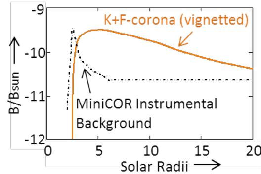
**Figure 7: The MiniCOR vignetted K- plus F-corona profile and the instrument background incident on the detectors are shown. The maximum instrument background is below the natural scene K- plus F-corona profiles over the entire field of view from 2.9-20 $R_s$ .**
