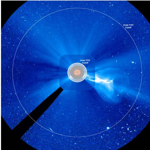
**Figure 1. The MiniCOR FOV covering 2.5-20  $R_s$  superimposed on the combined LASCO C2 & C3 FOV. The MiniCOR occulter (white semi-transparent circle) is comparable to the C2 occulter (2.5 vs. 2.2  $R_s$ ) but extends high resolution imaging into the C3 FOV. MiniCOR's plate scale is 19 arcsec/pixel compared to C3's 58 arcsec/pixel.**
