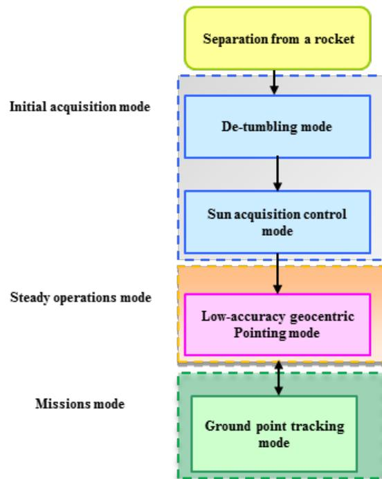
**Figure 2: Typical transition of attitude control modes**
