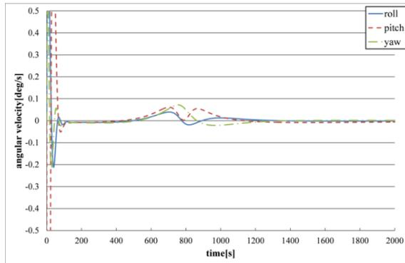
**Figure 8: Time history of the angular velocity errors**
