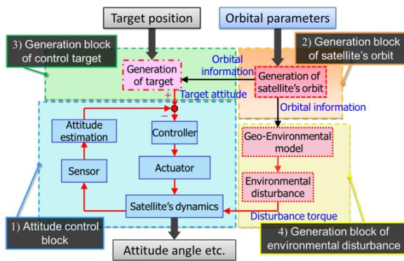
Figure 3: Block diagram of the simulator
