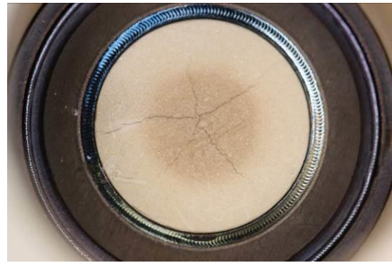
Figure 17: Cracks Propagating in Ceramic Insulation due to Thermal Expansion
