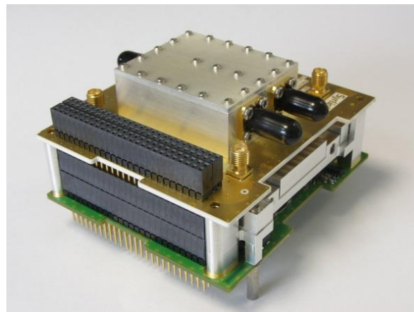
Figure 2 : EWC31 S band TT&C/ISL with a second diplexer configuration and integrated coupler
