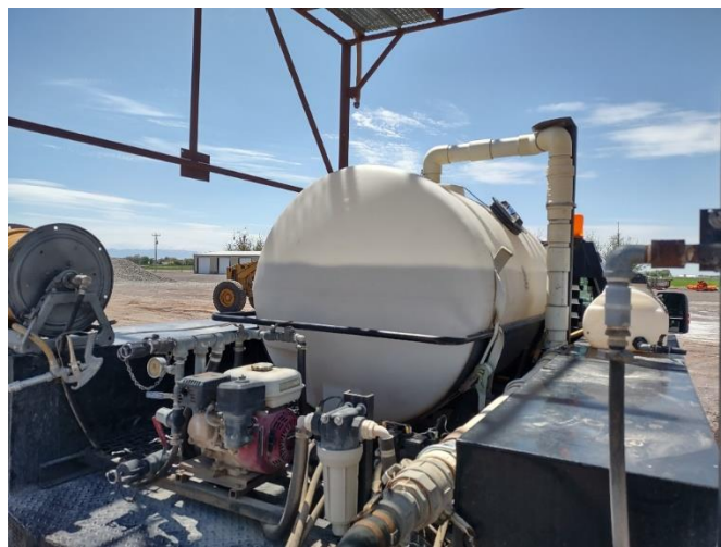
Figure 1. Spray Truck for Mixing and Applying Pesticides Over Large Areas
