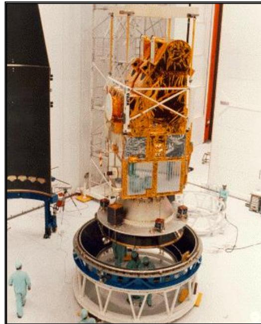
**Figure 2b ASAP Ring and Primary Payload (SPOT-1)**
