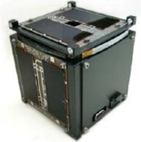
**Figure 4 Representative 1 Unit (1U) CubeSat**
