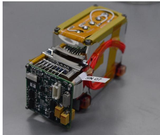
**Figure 8. Photograph of the AeroCube-OCSD-B & C propulsion module.**
