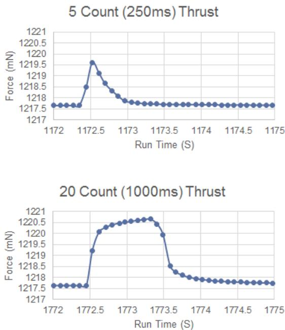
**Figure 9. Thrust measurements for 250 and 1000 ms pulse widths.**
