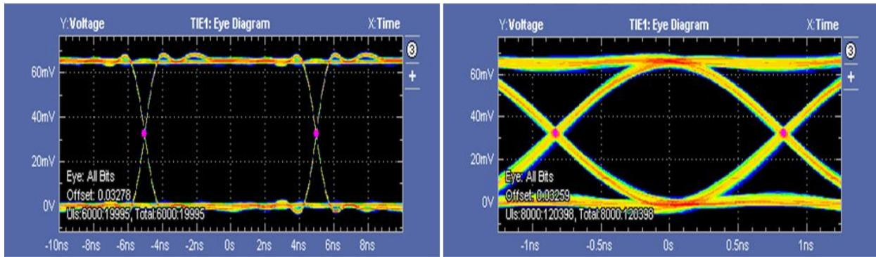
**Figure 7. Eye diagrams for the new laser transmitter at 100 Mbps (left) and at 622 Mbps (right).**
