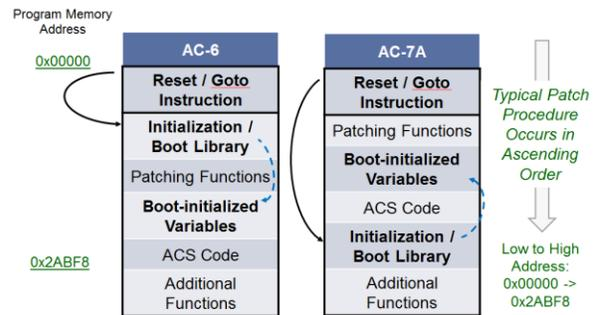
**Figure 10. Example memory maps for legacy (AeroCube-6) and OCSD-A (AC-7A) ACS processors.**
