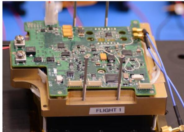
Figure 5. Downlink laser in the Pathfinder (AeroCube-OCSD-A).
