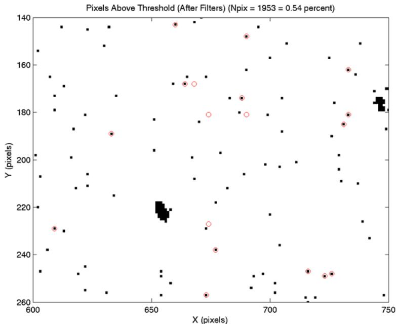
**Figure 4. Part of a processed stellar image, in negative form, from one of the star trackers.**
