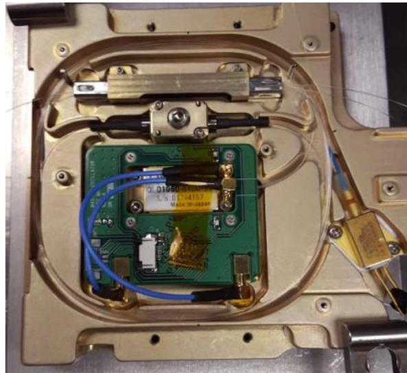
Figure 6. Downlink laser in the Demonstrators (AeroCube-OCSD-B and -C).
