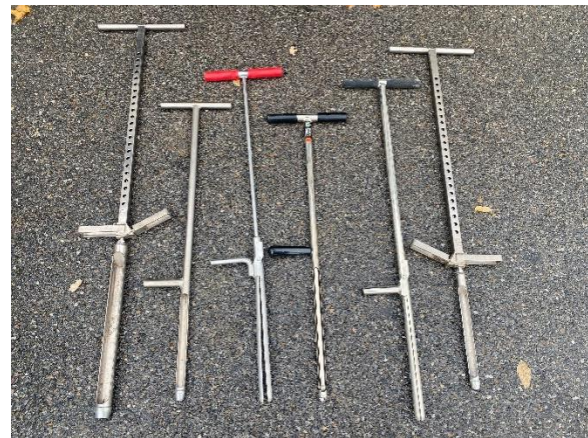
Figure 6. Examples of Soil Sampling Probe Options, Including Split Tube, Open Tube, Closed Tube With Slider, and Standard vs. Back-Saver Handles
