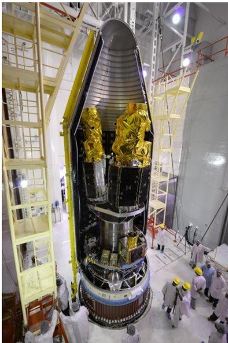
**Figure 2: DMC3 and Carbonite-1 satellites in shared PSLV-XL launch**
