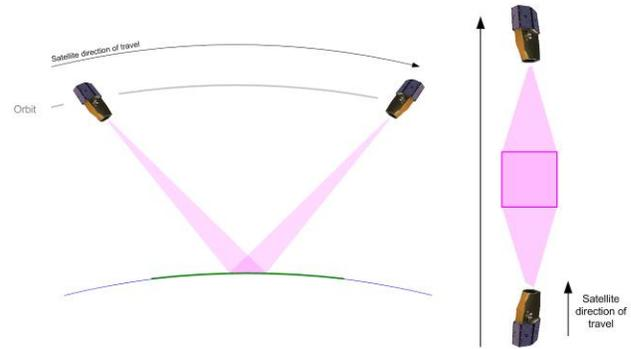
**Figure 3: Along-track stereo mode**
