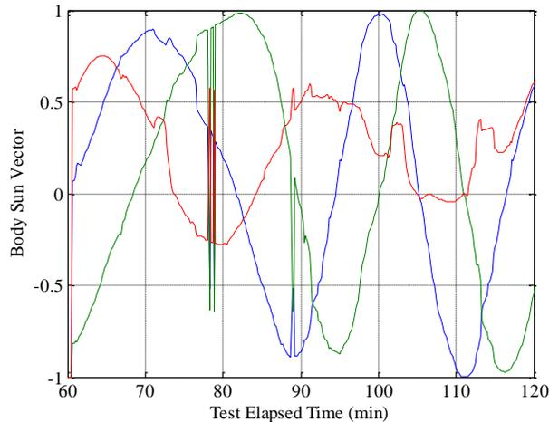
**Figure 5: Sun Vector Derived from Photocells**
