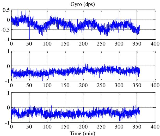
**Figure 6: Sample MEMS Gyro Performance**
