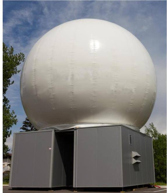
*Figure 2: Innovative two-layer thin membrane radome on test location.*
