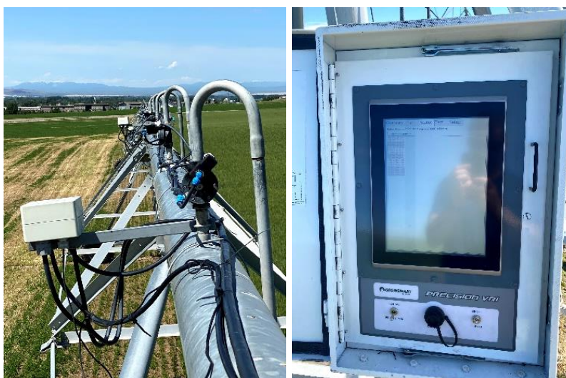
Figure 3. (left) Control Node Boxes and Valves on Each Pivot Drop, Required for Zone VRI; and (right) Add-on Panel to Existing Pivot, Enabling Zone VRI
