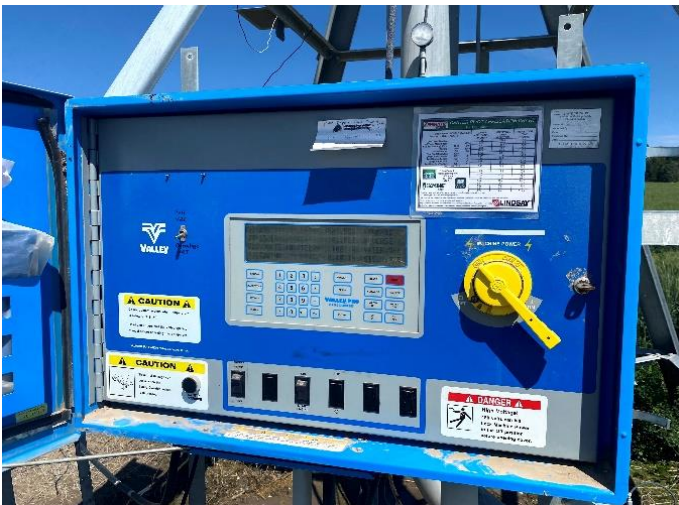
Figure 1. Pivot Panel With Speed Control Variable-Rate Irrigation Capability
