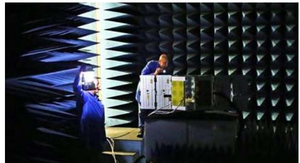
Figure 13 - CYGNSS Observatory during L-band noise floor testing
