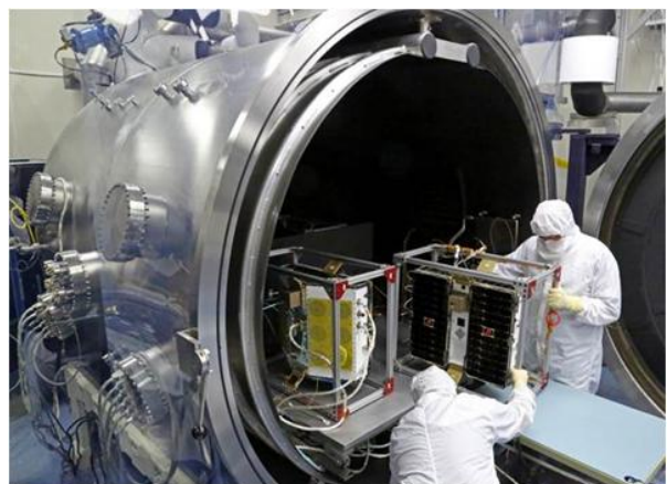
Figure 14 - CYGNSS observatory level thermal vacuum testing
