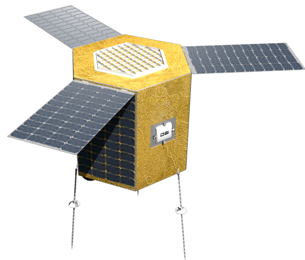
Figure 3: Prospector-1 Spacecraft – Depicting main solar panels, scanning antenna array, reaction control thrusters, and landing penetrator legs
