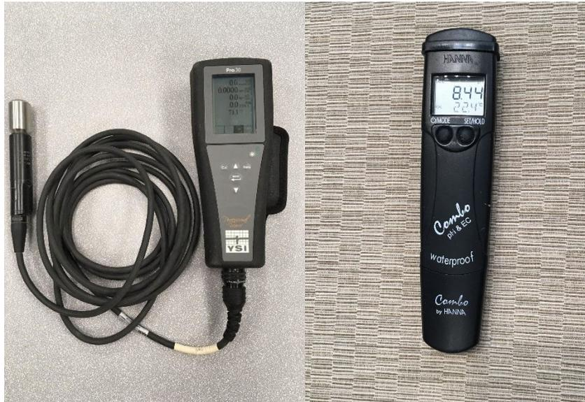
**Figure 8.** Example Photos of Handheld Water Quality Field Probes
