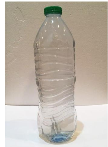
**Figure 10.** Water Sample in a Water Bottle, Triple-Rinsed in the Source Water Before Collection
