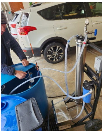
Figure 8. Reverse Osmosis System
