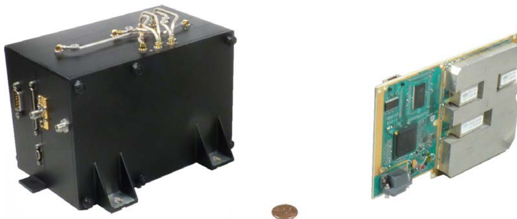
Figure 1: Comparison of the Van Allen Probes Frontier Radio (left) vs. FR Lite (right)
