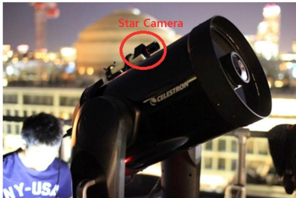
**Figure 2: Telescope and star camera.**
