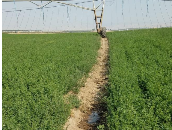
Figure 11. Dry and Shallow Wheel Track on a Pivot With a Mobile Drip Irrigation System
