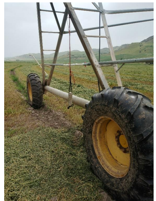
Figure 6. Polyacrylamide (PAM) Log Inside a Plastic Mesh Sack Hung Above the Wheel Track, Which Sprinkler Water Hits and Dissolves, Causing It to Drip Into the Wheel Rut
