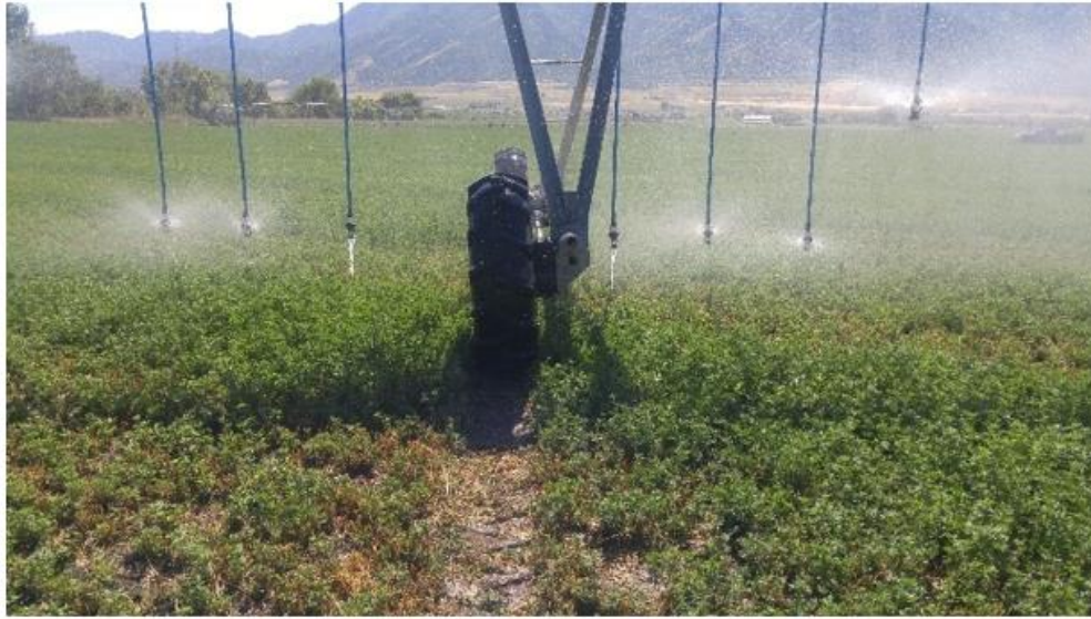
Figure 13. Low-Elevation Precision Application (LEPA) Style Sprinklers Used on Outlets Near the Wheel Tracks Can Keep Water Off the Track, and Bubbler Pads Can Also Prevent Water From Pooling in Tracks
