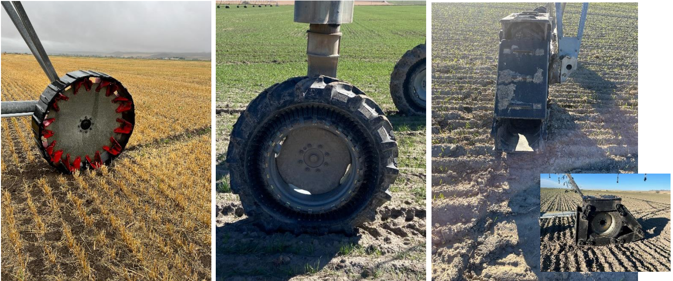
Figure 5. Examples of Pivot Tire Modification Examples, Including the NFTrax2.0 by Lindsay Corporation (left), the Irricup by Galileo Cupwheel (middle) and RAAFT by Polytech LLC (right, and insert)
