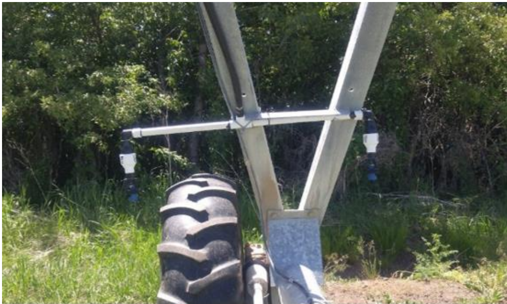
Figure 7. Dual Part-Circle Sprinkler System Mounted to a PVC Pipe Manifold, Developed and Tested by Utah State University
