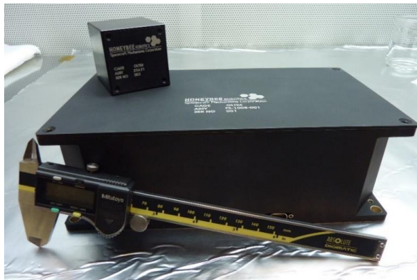
Figure 1: MicroSat Control Moment Gyros developed by Honeybee Robotics 1
