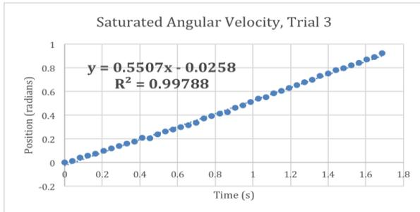
**Figure 3: Saturated angular velocity for inertia trial**
