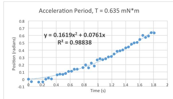
**Figure 5: Data from the acceleration period. The initial time and position of this period was subtracted from the raw data shown in figure 4.**
