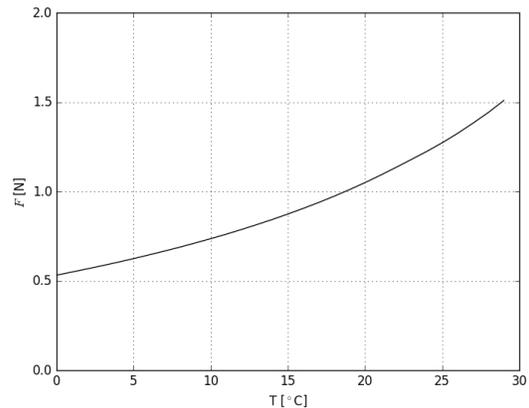
Figure 1: System thrust level varying with ambient temperature.
