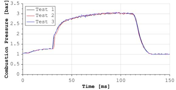
**Figure 4: Demonstrated repeatability in 3 minimum impulse bit pulses.**
