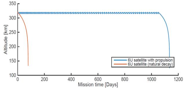
**Figure 6: Natural orbit decay of a 6U satellite vs extended mission using a HT-PM400.10 propelled 6U satellite. Atmospheric conditions representative for a mission begin in July 2017.**
