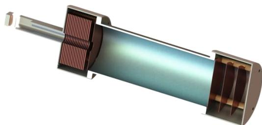
**Figure 3. The Mini-SUDA concept is a small version of EMFM's particle analyzer instrument. Sensor head (shown) integrates area-selectable target (at left), reflectron time-of-flight ion optics, and detector stack.**
