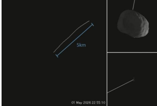
Figure 3: TetherSim Visualization of Asteroid De-Tumble. TetherSim allows for physics based analysis of tether and endbody dynamics.
