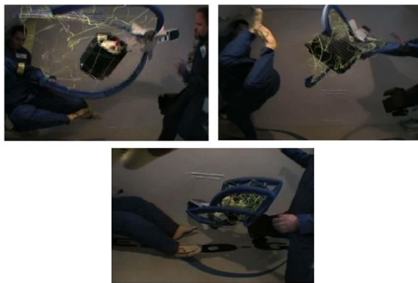
Figure 8: Zero-G Flight Test of GRASP Prototype. GRASP provides a scalable solution capable of capturing tumbling objects in microgravity.
