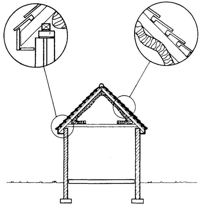
**Figure 5. A properly insulated roof will keep bats out.**
