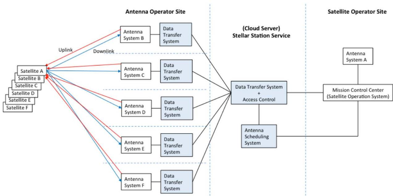
**Figure 9: Schematic of network operation**
