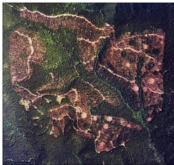
Figure 3. Overview of one replication of the Density Management Study right after installation. Note the range of densities, various gap and leave island sizes, and range of riparian buffer widths. Photo credit: Bureau of Land Management.
