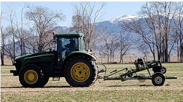
Figure 10. Gopher General-Used to Apply Aluminum Phosphide Into an Artificial Tunnel
