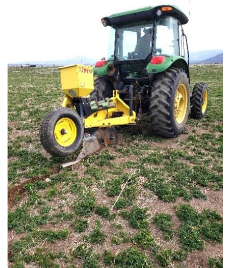
Figure 9. Burrow Builder Used to Apply Bait Into an Artificial Burrow
