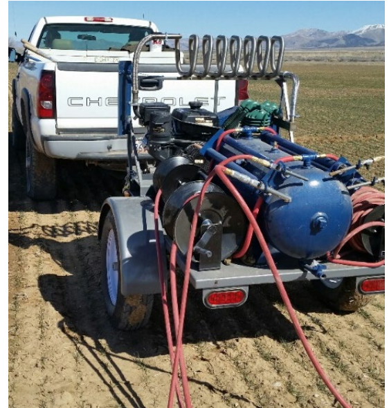
Figure 11. PERC Machine Used to Apply Carbon Monoxide Into Gopher Tunnel
