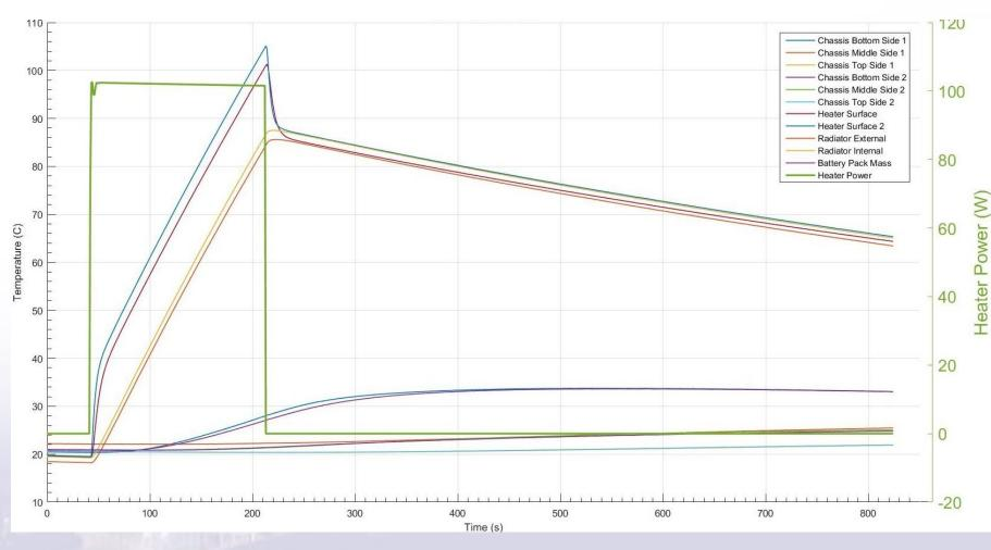
350 g heat sink provides ~3 minutes of run time with 100 W distribution at 20 C initial condition
