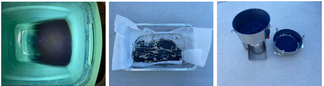
Figure 3. (left) Removing Water From Indigo Pigment, (center) Drying Indigo, and (right) Ground Indigo Powder
