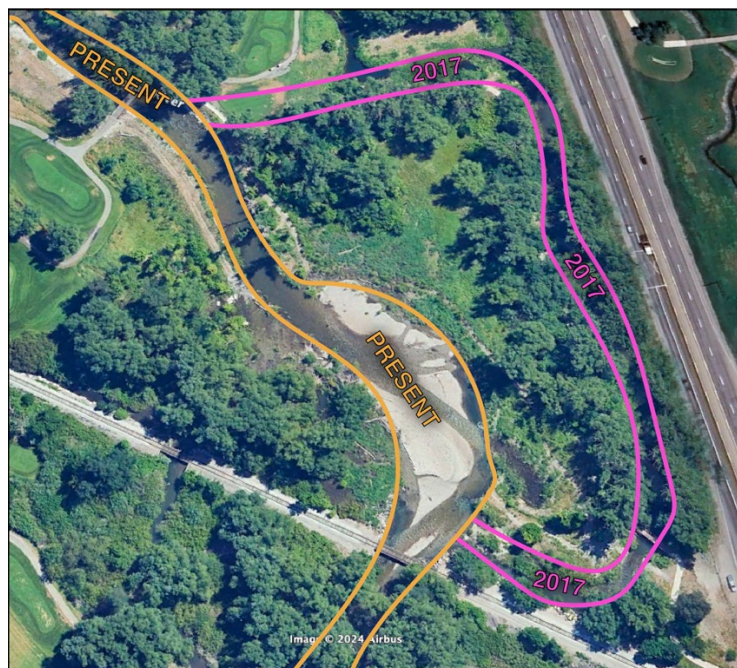
Figure 6. The Logan River's course in 2017 (pink) before the reroute and riffle pool creation, and the present-day route and riffle pool (orange).
