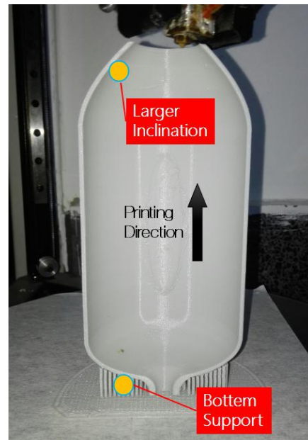
Figure 8: 1:1 Profile Model of the Steam Storage Tank in a Fused Deposition Modeling (FDM) Printer
