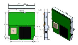
Figure 6: ThinSat Dimensions in Millimeters
