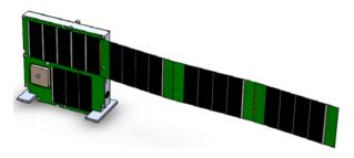
Figure 11: ThinSat Fanfold Solar Array
