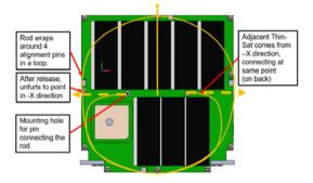
**Figure 12:Nitinol Wire Configuration**
