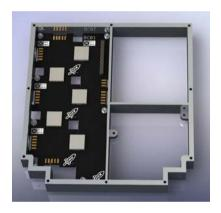
Figure 4: frame with X-Chip motherboard
