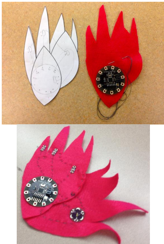
Figure 2. Romana's initial circuitry blueprint, in-process project, and completed felt patch with light sensor.
