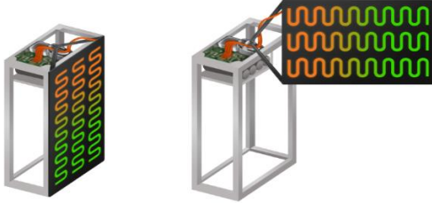
Figure 1 Left: Stowed Radiator system, Right: Deployed system
