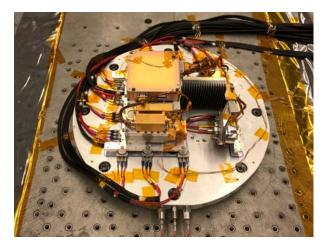
Figure 4: TEMPEST-D flight model radiometer instrument in vibration testing configuration at JPL
