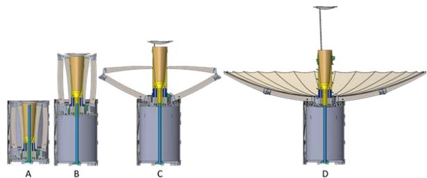
**Figure 4: The deployment sequence unfurls the 0.5m antenna from a 0.1m diameter cylinder.**
