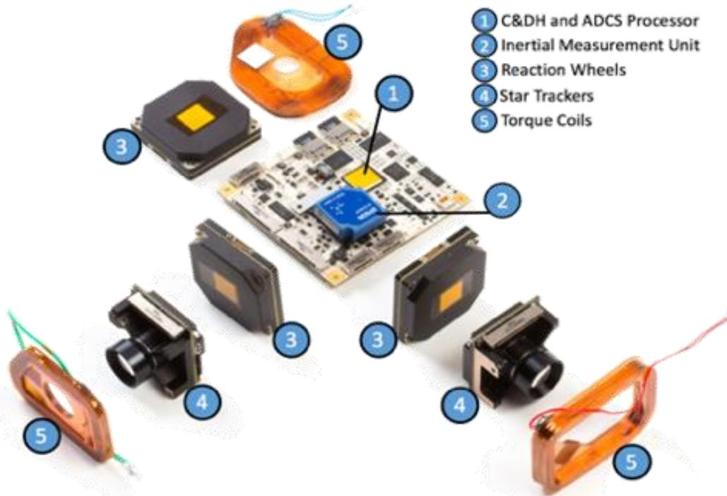
**Figure 5. An exploded view of the Tyvak avionics shows the Core Command and Data Handling and Attitude Determination and Control System. For RainCube, the torque coils are replaced with torque rods for improved torque authority at lower altitudes.**
