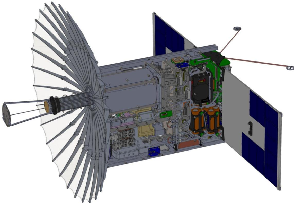
**Figure 6. No extra volume is wasted in the final pre-fabrication CAD rendering! The spacecraft is assembled by first installing the integrated radar (left), followed by the bus avionics (right), and finally closing out the system with remaining structure and deployable solar panels.**
