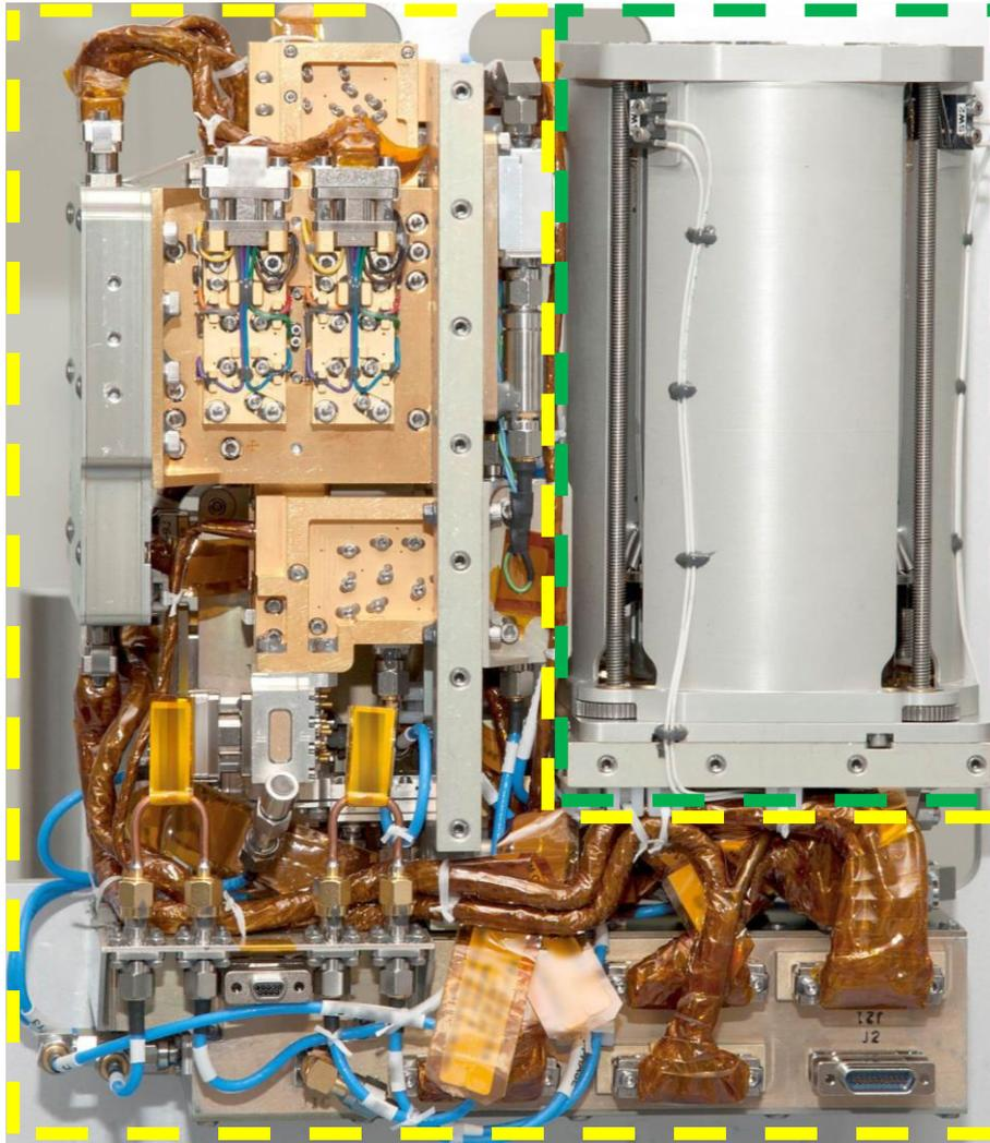
**Figure 2. The radar electronics (yellow) and deployable antenna (green) integrated into the flight chassis. The payload has undergone qualification vibe and t-vac testing at JPL.**
