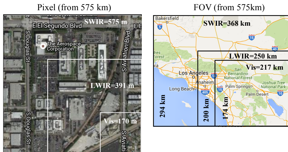
Figure 5: Pixel footprints and fields of view for the three CUMULOS cameras projected onto The Aerospace Corporation and the Los Angeles region. The cameras are co-boresighted.
