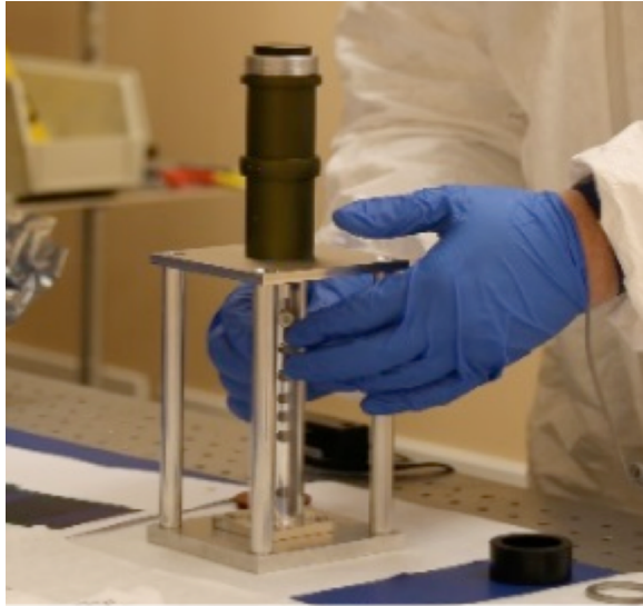
Figure 10: Assembly of optical telescope utilizing ground support equipment to ease installation
