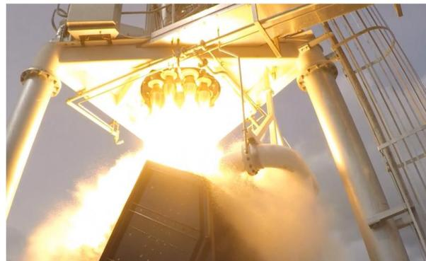
**Figure 3: Testing of 9 Rutherford Engines on Stage One**
