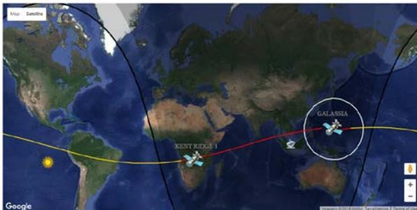
**Figure 2: Real-time Google Maps View with Satellite, Footprint, Primary Orbital Path, Ground Station, Sun Marker and Night Shadow Position Overlay**
