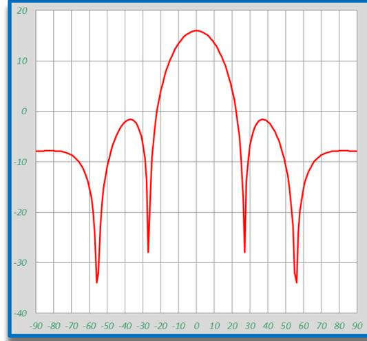
**Figure 7: Tower Antenna Gain pattern**
