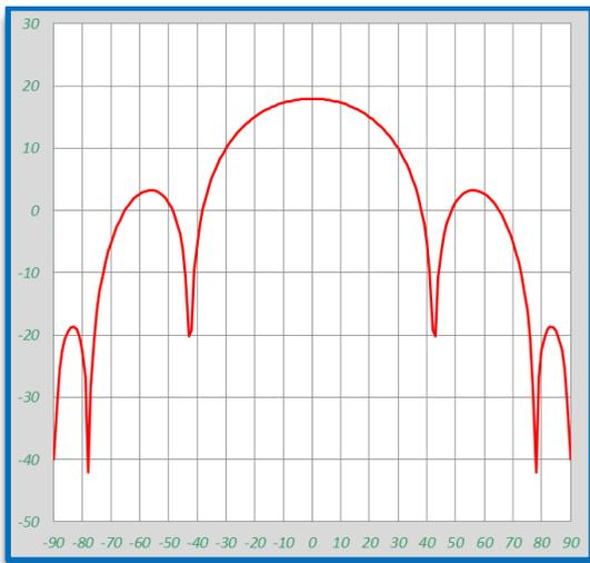
**Figure 6: Satellite Antenna Gain pattern**
