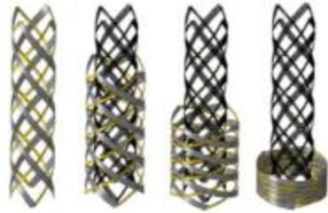
**Figure 5: Deployable Helical Antenna**
