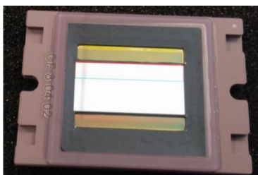
Figure 7: CMV12000 imager with integrated hyperspectral filter bank and panchromatic zone
