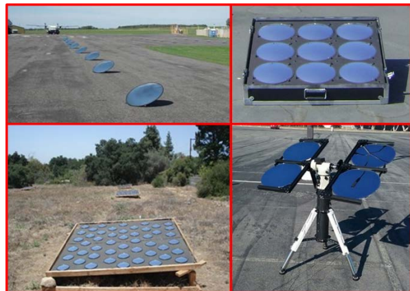
Figure 11. Examples of deployed SPARC spatial and radiometric calibration targets.
